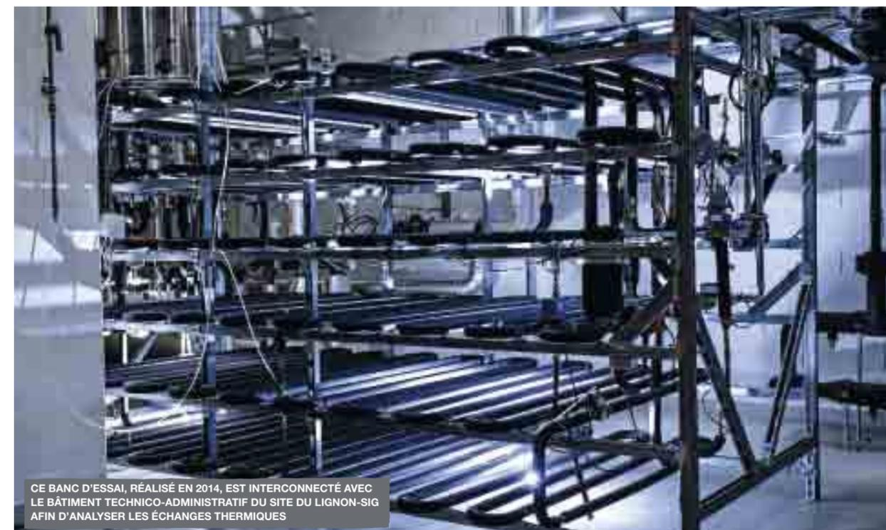
CE BANC D'ESSAI, RÉALISÉ EN 2014, EST INTERCONNECTÉ AVEC LE BÂTIMENT TECHNICO-ADMINISTRATIF DU SITE DU LIGNON-SIG AFIN D'ANALYSER LES ÉCHANGES THERMIQUES
